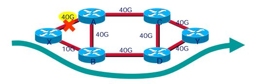
However, in this topology when optimization goal is to minimize bandwidth for single element failure conditions, if the demands from X→Y > 10G, TE cannot help - must upgrade link X→B
