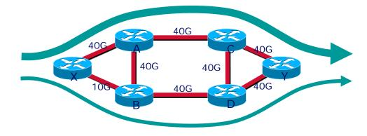
In this asymmetrical topology, if the demands from X→Y > 10G, traffic engineering can help to distribute the load when all links are working
