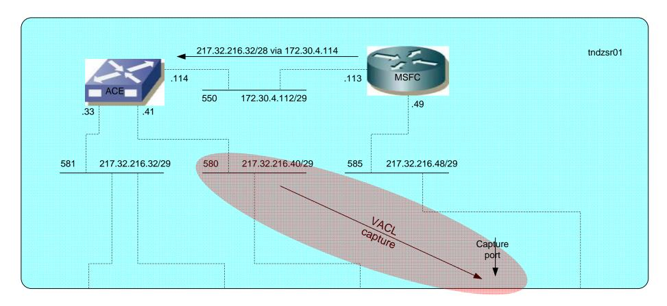
Using VLAN ACL (VACL) to capture traffic requires 4 basic steps:
