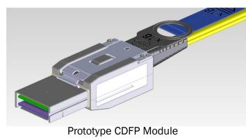
Optical Interface With Two 16 Fiber Ribbons (16 Transmit Fibers + 16 Receiver Fibers)
