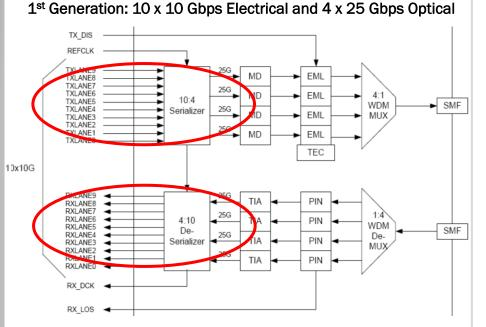
10 Gbps Electrical Signaling and 10:4 Gearbox Adds Complexity, Cost, Space, Power...
