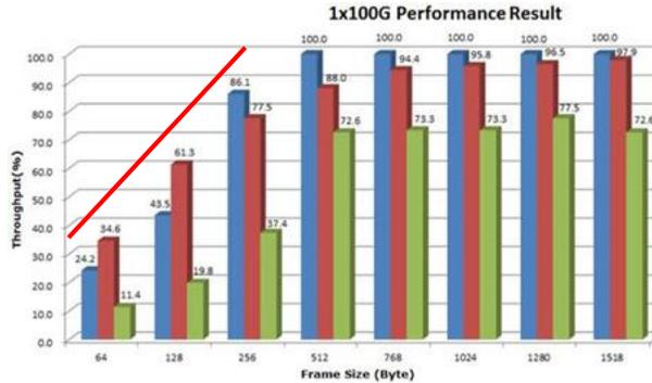
100G NIC comparison, using single Xeon E5-2658v4 @ 2.30GHz, 14 cores running DPDK software
