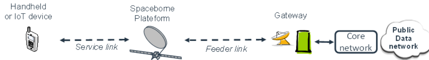
Figure 4.3-3A: Satellite access network with a service link operating in frequency bands below 6 GHz allocated to Mobile Satellite Services (MSS)
